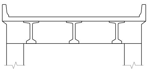
Figure 5-10: Indirect Support/Loading – Integral Pier Cap
